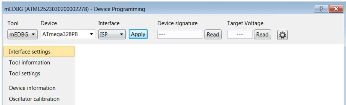
3. Select **Tool settings** and click on **Set target power switch off**, as shown below.
